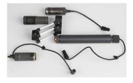
First install MKH8030 in the DMS clip, then the fig 8 and rear MKH8040. Adjust the coincidence of the two MKH8040 with the MKH8030 and secure with the screws M3x10 (cross recessed pan head screws with type Z)
